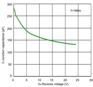
Fig 4. Capacitance vs. Reveres voltage
