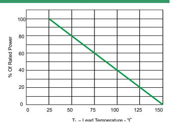
Fig 2.Power Derating Curve
