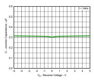
Fig 7. Capacitance vs. Reveres voltage
