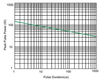
Fig 6. Non-Repetitive Peak Pulse Power vs. Pulse time
