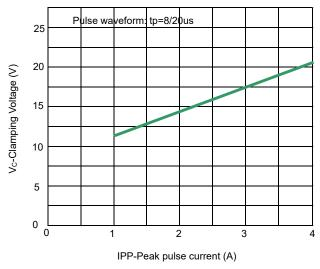
Fig 5. Clamping voltage vs. Peak pulse current
