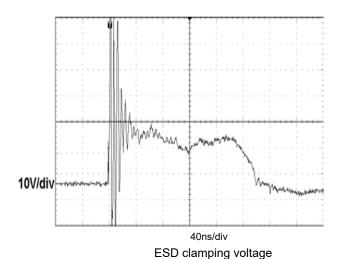
Fig 8. (IEC61000-4-2 +8KV contact)
