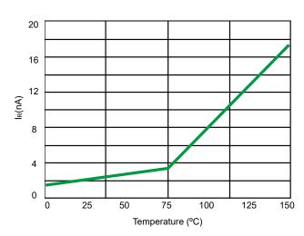
Fig 4. Typical Leakage Current vs. Temperature
