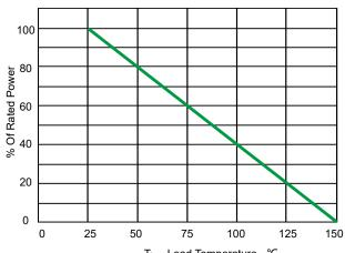
T<sub>1</sub> – I ead Temperature - °C Fig 2.Power Derating Curve
