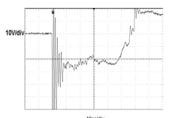
40ns/div ESD clamping voltage Fig 9. (IEC61000-4-2-8KV contact)
