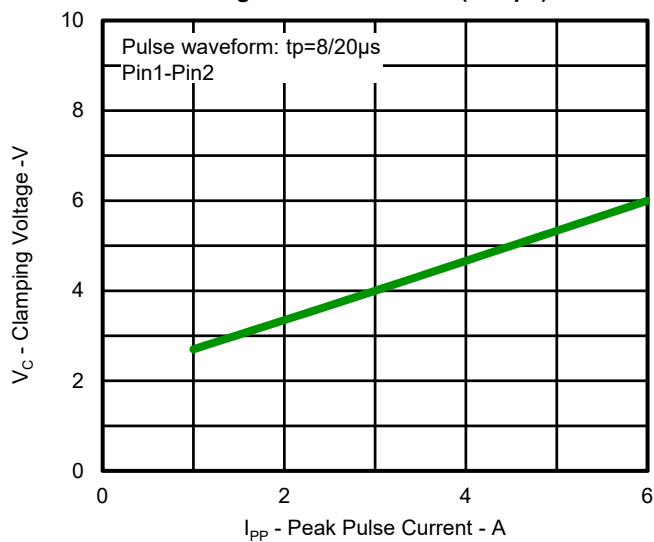
Fig.3 Clamping Voltage vs. Peak Pulse Current
