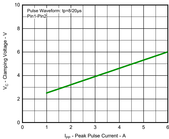
Fig 3. Clamping Voltage vs. Peak Pulse Current
