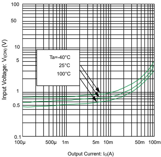
Fig 1. Input Voltage vs. output current
