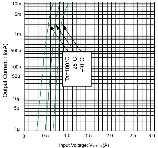
Fig 2. Output current vs. input voltage
