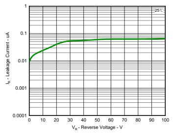
Fig 3.Typical Reverse Characteristics
