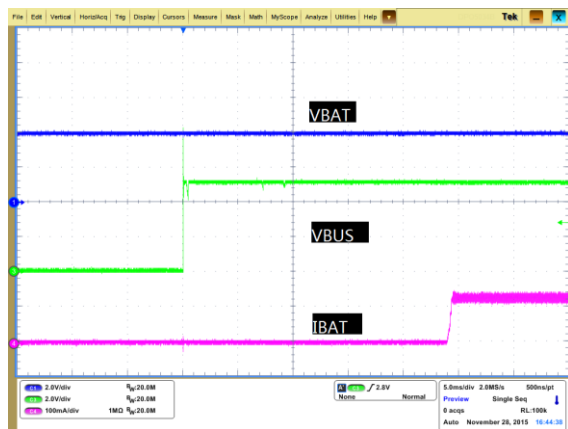
Figure 9. Auto-Charge Startup at V_{BUS} Plug-in, I_{INLIM}=100mA , V_{BAT}=3.9V
