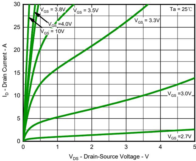
**Fig.1 Output Characteristics**
