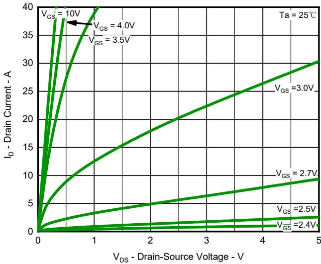
**Fig.1 Output Characteristics**
