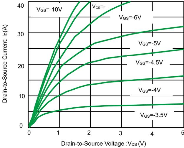
Fig 1. Output Characteristics
