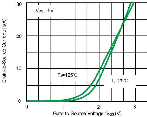
Fig 3. Transfer Characteristics
