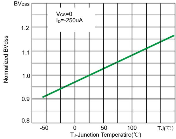
Fig 8. BV<sub>DSS</sub> vs Junction Temperature
