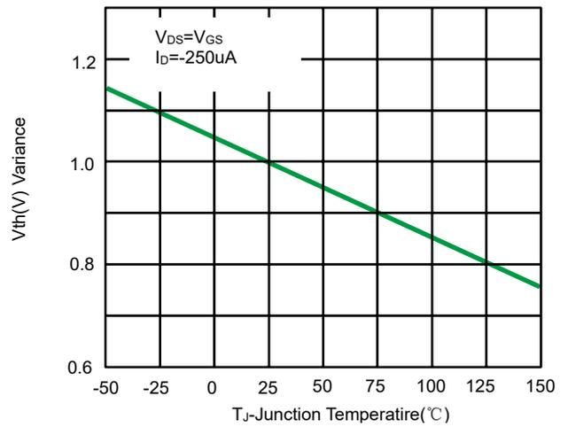
Fig 10. V<sub>GS(th)</sub> vs Junction Temperature
