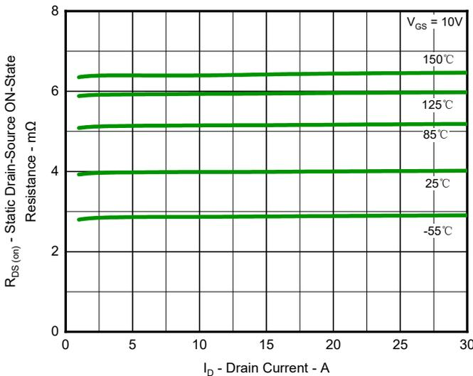
Fig.3 Typical On-Resistance vs Drain Current and Temperature
