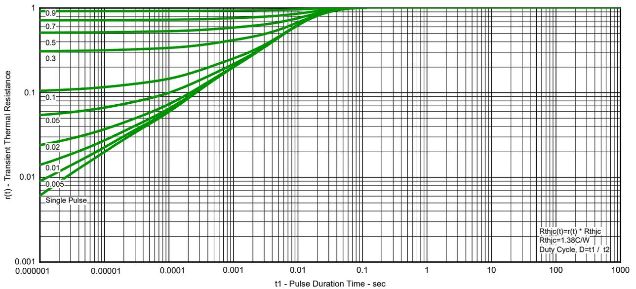
Fig.7 Transient Thermal Resistance
