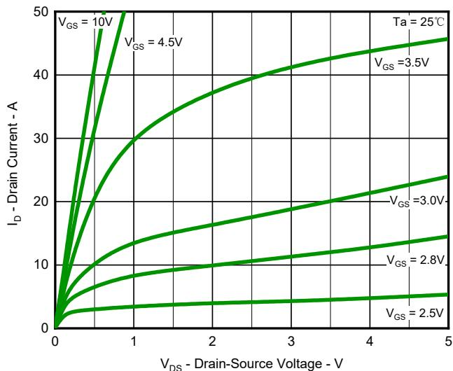
**Fig.1 Output Characteristics**
