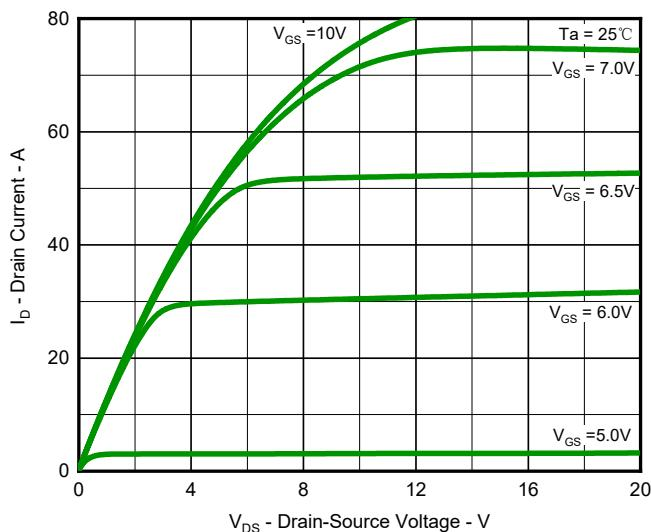
Fig.1 Output Characteristics
