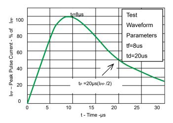
Fig 1.Pulse Waveform
