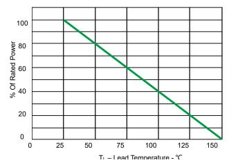
Fig 2.Power Derating Curve
