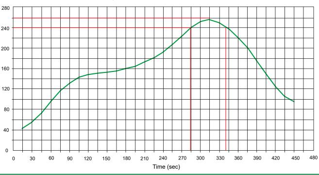
Peak Temp=257°C, Ramp Rate=0.802deg. °C/sec
