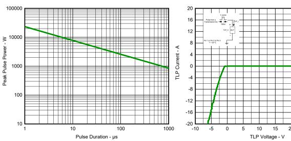
Fig 5. Non Repetitive Peak Pulse Power vs. Pulse time
