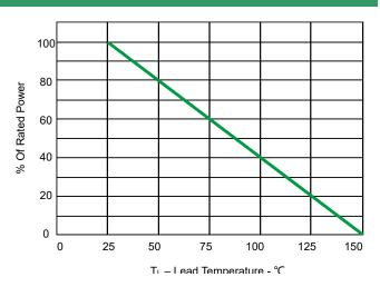
Fig 2.Power Derating Curve
