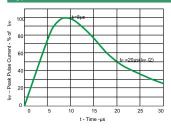
Fig 1.Pulse Waveform
