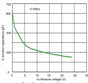
Fig 4. Capacitance vs. Reveres voltage
