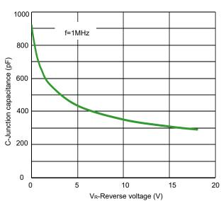
Fig 4. Capacitance vs. Reveres voltage
