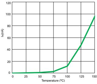
Fig 6. Typical Leakage Current vs. Temperature
