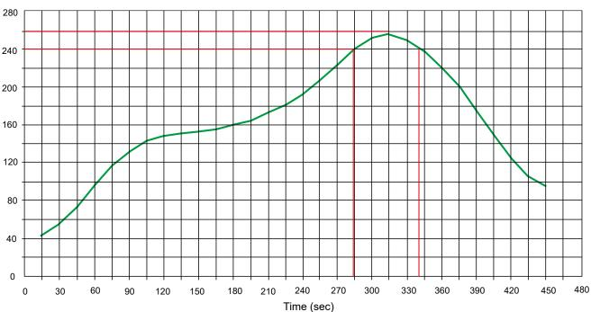
Peak Temp=257°C, Ramp Rate=0.802deg. °C/sec
