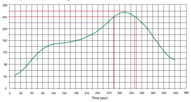
Peak Temp=257°C, Ramp Rate=0.802deg. °C/sec
