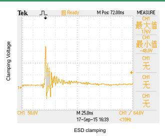
Fig 7 (8kV contact discharge per IEC61000-4-2)
