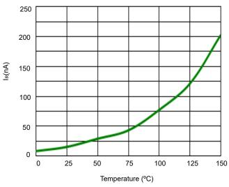
Fig 6.Typical Leakage Current vs. Temperature
