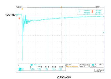
Fig 8. ESD clamping voltage (IEC61000-4-2 -8KV contact)
