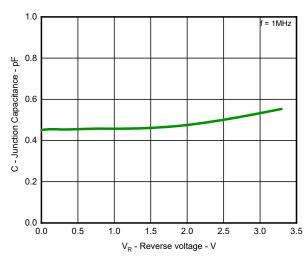
Fig 4. Capacitance vs. Reveres voltage
