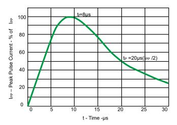
Fig 1.Pulse Waveform
