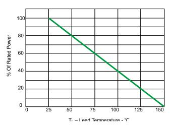
Fig 2.Power Derating Curve
