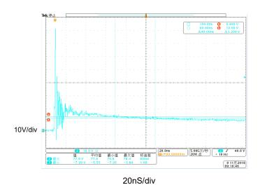
Fig 7. ESD clamping voltage (IEC61000-4-2 +8KV contact)
