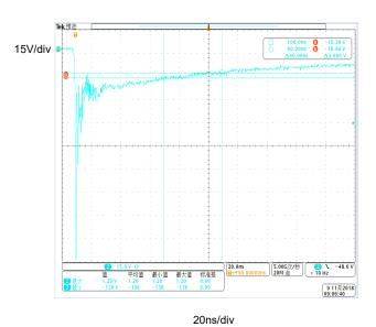
Fig 8 ESD clamping voltage (IEC61000-4-2-8kv contact )
