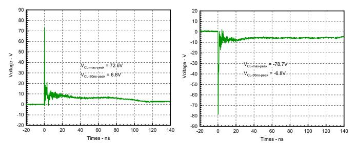
Fig 7. Clamping Voltage at IEC61000-4-2 +8kV Pulse Waveform
