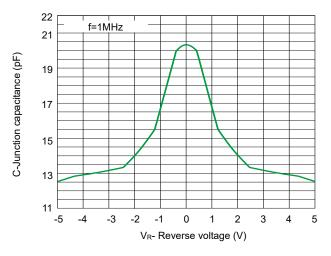
Fig 3. Capacitance vs. Reveres voltage
