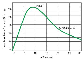
Fig 1.Pulse Waveform
