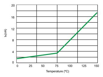
Fig 4. Typical Leakage Current vs. Temperature
