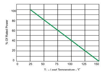
Fig 2.Power Derating Curve
