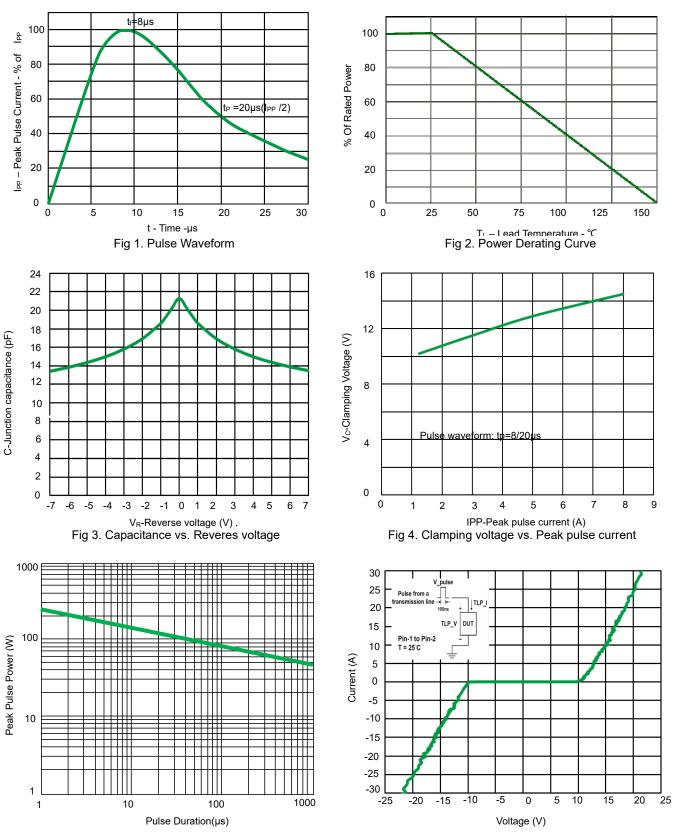
Fig 5. Non-Repetitive Peak Pulse Power vs. Pulse time
