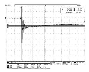
Fig 7. ESD clamping voltage (IEC61000-4-2 +8kV contact)
