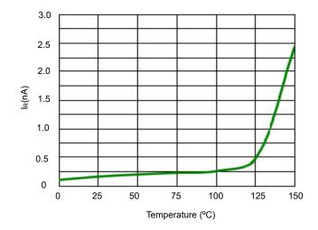
Fig 5.Typical Leakage Current vs. Temperature
