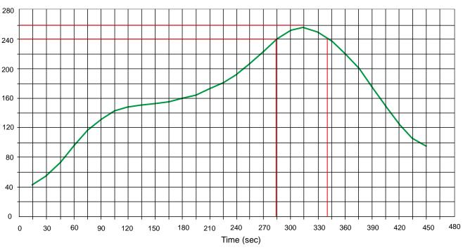
Peak Temp=257°C, Ramp Rate=0.802deg. °C/sec
