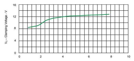
Fig.1 Typical Clamping Voltage VS Peak Pulse Current for PESDLC363T5VU
