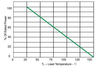
Fig 3.Power Derating Curve
