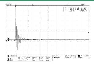
Fig 7. ESD clamping voltage (IEC61000-4-2 +8kV contact)
