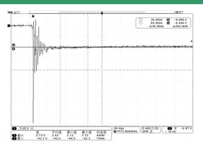
Fig 8. ESD clamping voltage (IEC61000-4-2-8kV contact)
