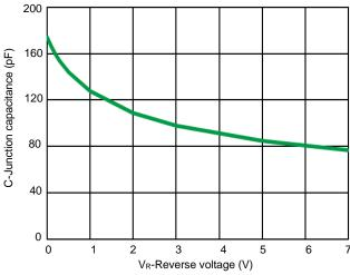
Fig 6. Capacitance vs. Reveres voltage
