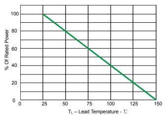
Fig 2.Power Derating Curve
