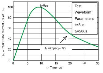
Fig 1.Pulse Waveform
