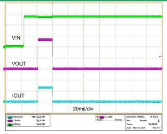
Power on Response(Rout=10 $\Omega$ ,R<sub>ILIM</sub>=1k $\Omega$ )
