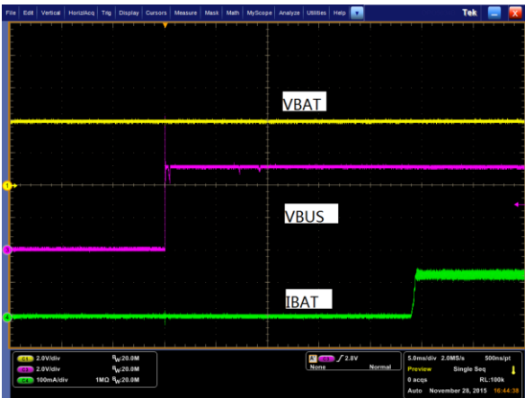
Figure 9. Auto-Charge Startup at V_{BUS} Plug-in, I_{INLIM}=100mA , V_{BAT}=3.9V
