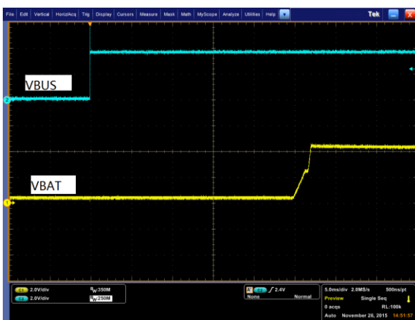
Figure 15. No Battery at V_{BUS} Power-up
