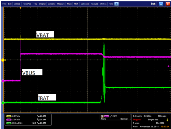
Figure 11. Auto-Charge Startup with 300mA Limited Charger/Adaptor, I_{INLIM}=500mA , V_{BAT}=3.9V
