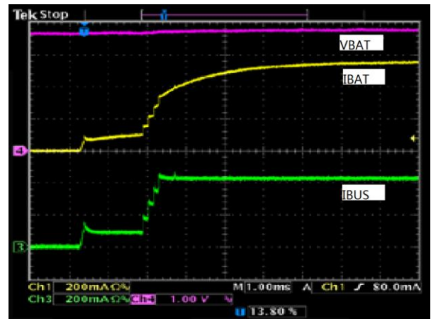
Figure 12. Charger Startup with HZ_MODE Bit Reset, I_{INLIM}=500mA , I_{OCHARGE}=956mA , O_{REG}=4.2V , V_{BAT}=3.6V
