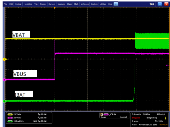
Figure 10. Auto-Charge Startup at V_{BUS} Plug-in, I_{INLIM}=500mA , V_{BAT}=3.9V
