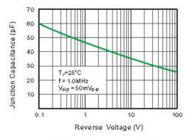
Fig.5 Typical Junction Capacitance
