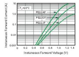
Fig.4 Typical Forward Characteristics
