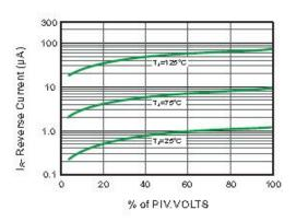
Fig.3 Typical Reverse Characteristics
