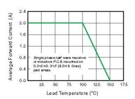
Fig.2 Maximum Average Forward Current Rating
