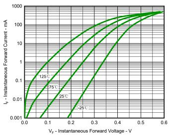
Fig.1 Typical Forward Characteristics
