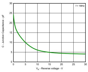
Fig 3.Capacitance vs. Reveres voltage
