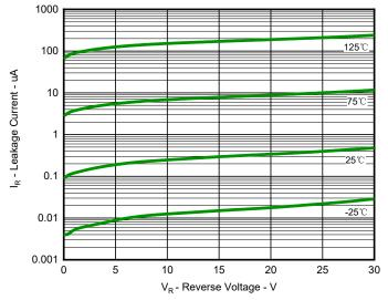
Fig 2.Leakage Current
