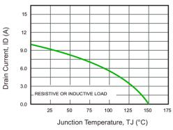
Fig.12 Drain Current vs. Junction Temperature
