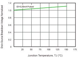
Fig.6 Breakdown Voltage vs. Junction Temperature
