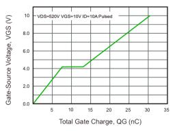
Fig.3 Gate Charge Characteristics
