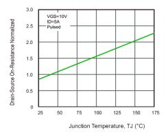
Fig.5 Drain-Source On-Resistance vs. Junction Temperature
