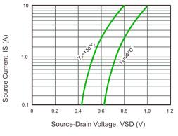
Fig.8 Source Current vs. Source-Drain Voltage
