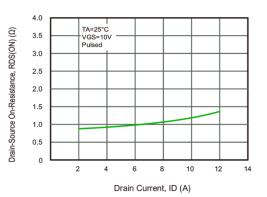
Fig.10 Drain-Source On-Resistance vs. Drain Current
