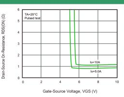
Fig.2 Drain-Source On-Resistance vs. Gate-Source Voltage
