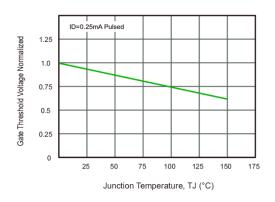
Fig.7 Gate Threshold Voltage vs. Junction Temperature
