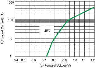
Fig 1.Typical Forward Voltage
