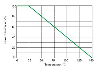
Fig 4.Steady State Power Detating
