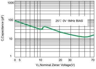
Fig 2. Typical Capacitance
